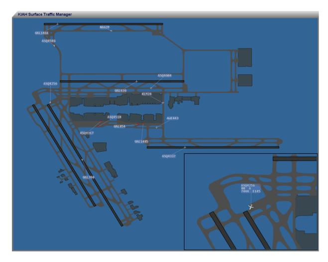
I2M Systems Inc. Surface Traffic Management (I2-STM) is designed to enhance the efficiency and safety of air traffic operations. It allows maximization of the efficiency of the aerodrome environment by providing the controller detailed situational awareness data in low visibility conditions. I2-STM also enhances safety by providing customizable automated "safety nets" which provide alerts to controllers to prevent potentially imminent incidents.
