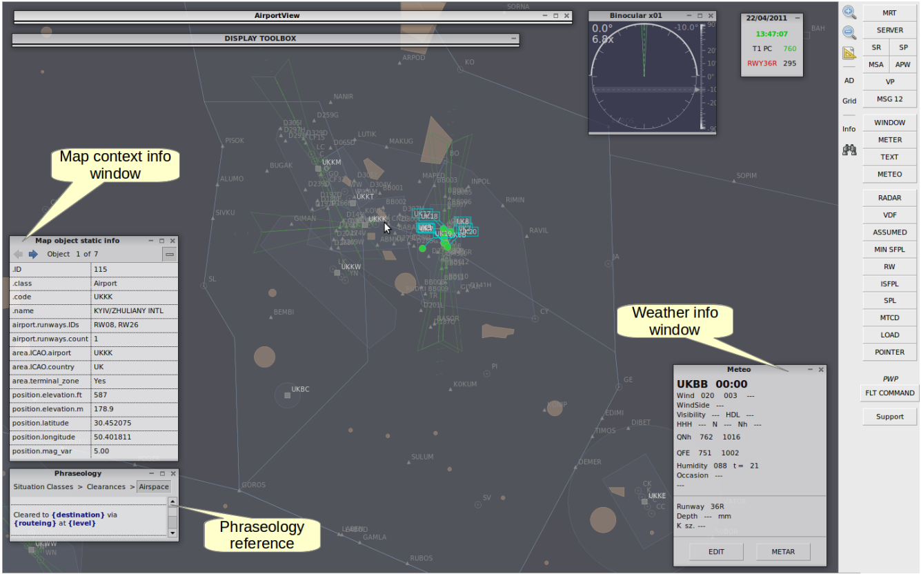
Picture 2 – Main Surveillance Display: auxiliary information windows
